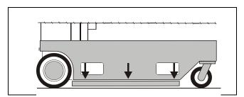
Figure 2-2. Pot-Hole-Protection Bars Lowered.
