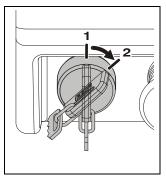
At the Platform Control Console - Set the On/Off Key Switch to the ON position (2) to operate machine.
