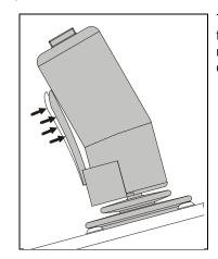
The Function Enable lever on the front of the joystick control, must be engaged and held in during any joystick operation.
