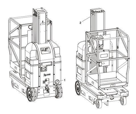
Figure 5-2. Location of Lubrication Points (See Table 5-5)
