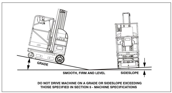
**Figure 3-4. Machine Operating Specifications**
