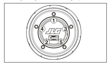
Figure 5-1. Wheel Lug Nut Tightening Sequence
