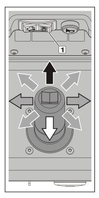
Activate the Drive Mode using the Drive/Lift Mode Selector switch.
