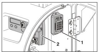
Figure 3-7. PSL<sup>™</sup> Switch & Ground Control Station Locations - At Rear of Machine.
