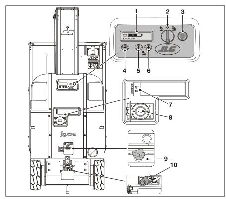
Figure 3-1. Ground Control Station. (Machine Rear View)
