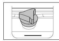
FILL TO LINE on Hydraulic Reservoir indicates the proper level for hydraulic oil.
