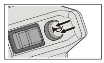
When the machine is powered on, pressing this button will sound the Horn.
