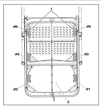
Figure 3-9. OSS Transducer Sensor Array Location.
