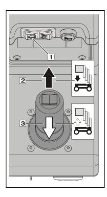
Activate the Lift Mode using the Drive/Lift Mode Selector switch.
