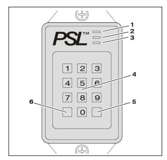
Figure 3-8. PSL<sup>™</sup> Switch Controls & Indicators.
