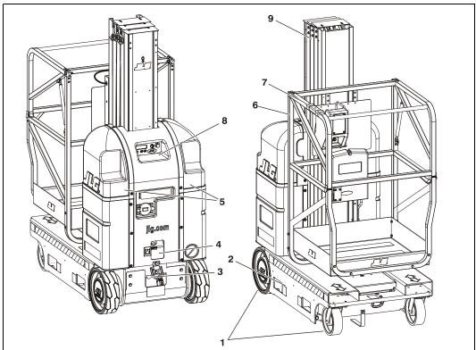
Figure 2-1. Daily Walk-Around Inspection for MVL/MSP Machines.
