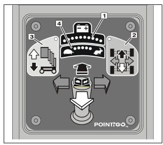
Figure 3-3. Platform Control Display Panel.
